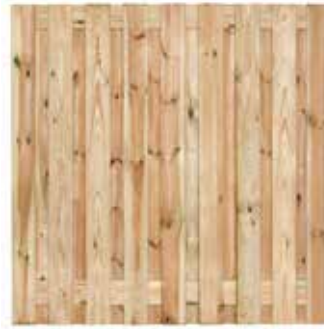
8.11180 Vasse 180 - Garden Fence H180xW180cm 17 planks of D1.6xW14.0cm Intermediate slat: D1.6xW14.0cm Planed, impregnated pine, Stainless steel screwed
