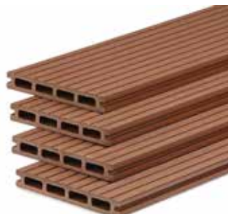
37.5550 Premium composite 2.1x15.0x400cm, redwood Coloured through and through, 100% recyclable, 60% wood / 40% synthetic, underside smooth planed, top side rough relief
