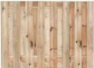
8.10130 Coevorden 130 - Garden Fence H130xW180cm 15 planks of D1.6xW14.0cm Intermediate slat: D1.6xW14.0cm Planed, impregnated pine, Stainless steel screwed
