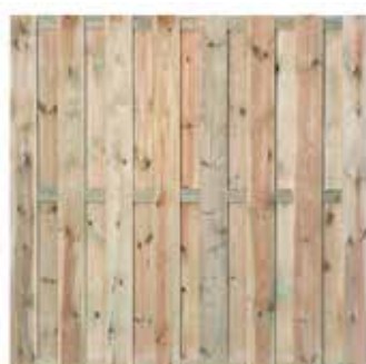
8.14184 Uden - Garden Fence H180xW180cm 15 planks of D1.5xW14.0cm Intermediate slat: D1.5xW7.0cm Planed, impregnated pine, Stainless steel screwed
