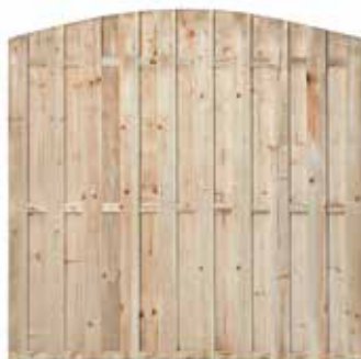
8.14180 Aalsmeer - Garden Fence H180xW180cm 19 planks of D1.0xW10.0cm Intermediate slat: D1.5xW5.0cm Rough, impregnated pine, stapled
