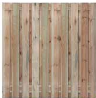
8.14186 Haaksbergen - Garden Fence H180xW180cm 19 planks of D1.5xW14.0cm Intermediate slat: D1.5xW14.0cm Planed, impregnated pine, Stainless steel screwed
