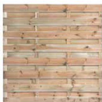
8.14185 Erica - Garden Fence H180xW180cm 15 planks of D1.6xW14.0cm Intermediate slat: D1.6xW7.0cm Planed, impregnated pine, Stainless steel screwed
