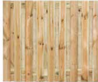
8.11150 Vasse 150 - Garden Fence H150xW180cm 17 planks of D1.6xW14.0cm Intermediate slat: D1.6xW14.0cm Planed, impregnated pine, Stainless steel screwed
