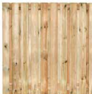
8.14190 Venray - Garden Fence H180xW180cm 19 planks of D1.7xW14.0cm Intermediate slat: D1.7xW14.0cm Planed, impregnated pine, Stainless steel screwed
