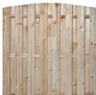
8.14182 Den Haag - Garden Fence H180xW180cm 15 planks of D1.5xW14.0cm Intermediate slat: D1.5xW7.0cm Planed, impregnated pine, screwed
