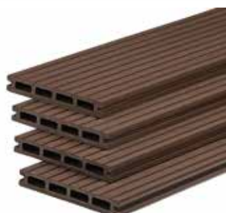
37.5570 Premium composite 2.1x15.0x400cm, coffee Coloured through and through, 100% recyclable, 60% wood / 40% synthetic, underside smooth planed, top side rough relief
