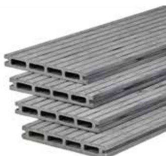
37.5580 Premium composite 2.1x15.0x400cm, classic grey Coloured through and through, 100% recyclable, 60% wood / 40% synthetic, underside smooth planed, top side rough relief
