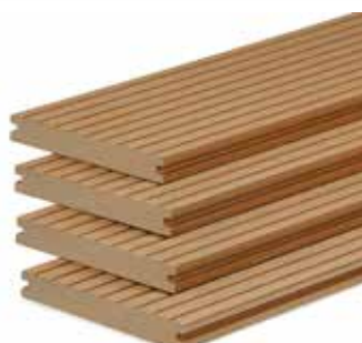
37.5652 Excellent solid composite 2.0x14.0x400cm, natural Coloured through and through, 100% recyclable, 60% wood / 40% synthetic, underside smooth planed, top side rough relief
