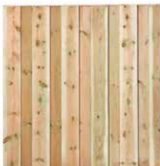
8.80086 Twente - Garden Fence H180xW180cm 11 planks of D1.8xW20.0cm Intermediate slat: none Fitted with upper and lower slats Planed, impregnated pine, Stainless steel screwed
