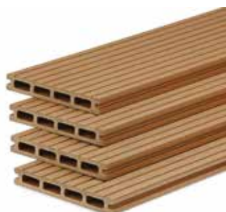
37.5560 Premium composite 2.1x15.0x400cm, natural Coloured through and through, 100% recyclable, 60% wood / 40% synthetic, underside smooth planed, top side rough relief
